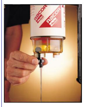
If you change over to E10 from non-ethanol gas, you should check for water in the water separating fuel filter. Carry spare filter elements, as ethanol is a solvent that loosens gunk in the fuel system.
